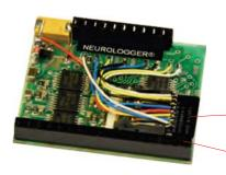
8 differential neurophysiological channels (EEG, ECG, EOG, EMG) three of which can be used for 3-D accelerometer 5.31 g recorder weight + ~9 g typical battery Total weight about 15 g without enclosure
