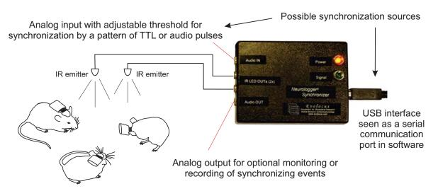
Standard serial interface is supported in Matlab, Labview, Python and all classical programming languages. We provide Matlab examples illustrating interaction with Neurologger Synchronizer. Analog input with adjustable threshold also can be used with a push button. Pressing on this button will initiate transmission of a predefined pattern of IR pulses to the Neurologgers. Software for conversion of Neurologger data to Matlab and other environments is provided.
