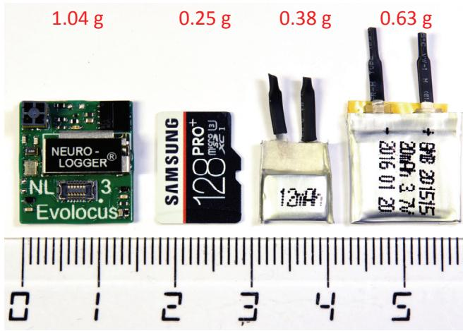
**Figure 2 |** Neurologger 3, an example of its memory (Samsung 128 GB Micro SDXC) and two examples of its battery. Batteries of different capacities can be used depending on desired record duration. Two examples of batteries of different weight/capacity are shown. The logger needs only one battery. Note that the duration of record is usually limited by the battery and not by the memory size.
