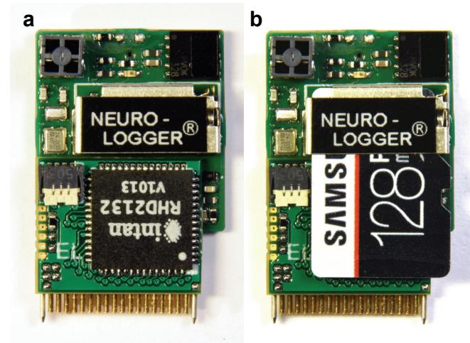
**Figure 3 |** Neurologger 3 with its headstage and memory. To record neuronal activity the neuronal headstage should be attached to the processor module how it is shown in this picture (a). The 32-channel headstage with Hirose connector is placed at the bottom side (invisible). Then, the memory card is placed above the headstage (b). This combination weighs 1.73 g.
