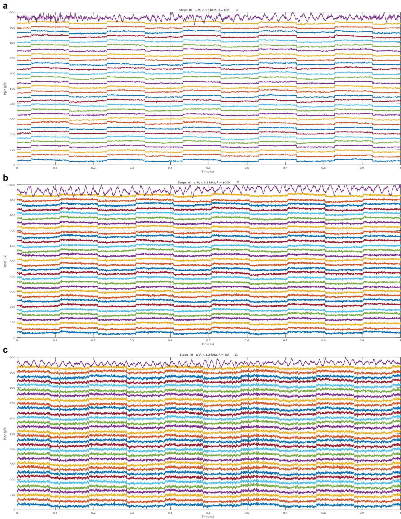
**Figure 6** | Noise and electromagnetic disturbances in the Neurologger 3 when a sequence of 10  $\mu\text{V}$  peak-to-peak rectangular pulses was given to the input of the logger through 10  $\text{k}\Omega$  (a), 100  $\text{k}\Omega$  (b) or 1  $\text{M}\Omega$  (c) resistors. All other conditions are identical to the conditions of the record in the Fig. 5.
