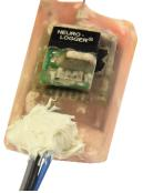
Water-proof ECG recorder for marine birds IR receiver is replaced by magnetic sensor. Putting permanent magnet in the vicinity of the sensor creates a label in the logger record. Memory 1 GB, rechargeable battery 3.7V, 240 mAh. The battery is sufficient for 4 days. Total weight of encapsulated logger 20 g.
