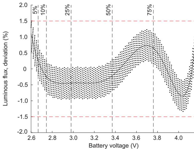
Solid black line shows luminous flux approximation error. It is below 1%. Dotted cloud around this line ( $\pm 0.5\%$ ) represents discretization error caused by 1% step of power adjustment. The total error is always below 1.5% in the displayed range of battery voltages.
